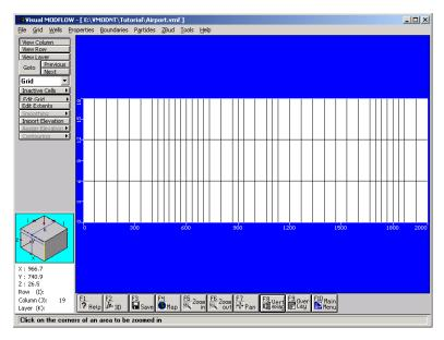
From the figure you can see that each layer has a uniform thickness across the entire cross-section. However, nature rarely provides us with geology that conforms to flat horizontal layering with uniform layer thickness.
