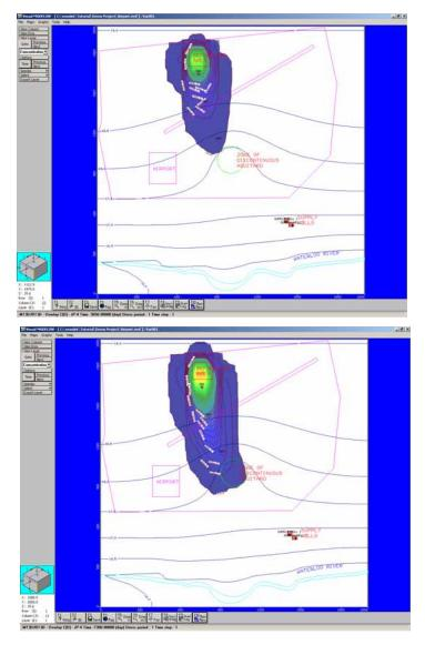
After **3650** days (10 years) of simulation time it is clear that the plume has migrated to the 'hole' in the aquitard.
