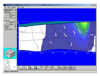
This figure shown the plume has migrated into the lower aquifer at a concentration above the action level and will eventually threaten the pumping wells. To see the plume in the lower aquifer,
