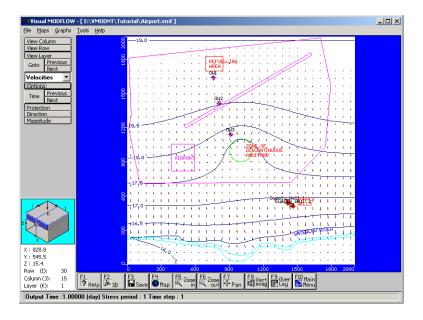
By default the color scheme for the velocity vectors is: **red** is outward (i.e. up when viewing by layer), **blue** is inward (i.e. down when viewing by layer), and **green** is parallel to the plane (i.e. horizontal when viewing by layer).
