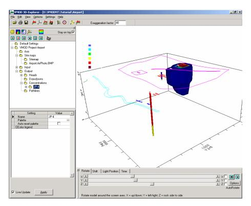
Notice that the concentration isosurface is clipped where the isosurface meets the water table. 3D-Explorer has built-in logic that removes concentration isosurfaces above the water table.
