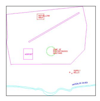
The municipal well field consists of two wells. The east well pumps at a constant rate of 550  $\rm m^3/day$ , while the west well pumps at a constant rate of 400  $\rm m^3/day$ . Over the past ten years, airplane fuel has periodically been spilled in the refuelling area and natural infiltration has produced a plume of contamination in the upper aquifer. This tutorial will guide you through
