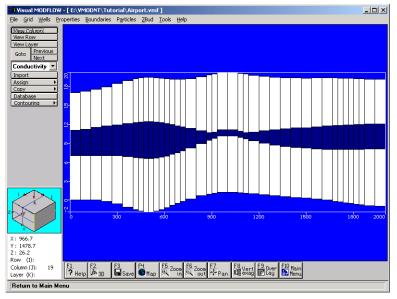
The upper aquifer, aquitard, and lower aquifer units should be plainly visible by the different colors of the Conductivity property zones, as shown in the previous figure (viewing column 19).
