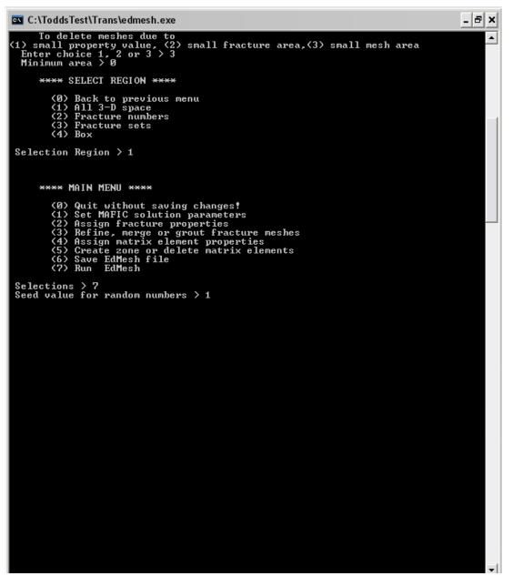
After this step, hitting enter, EdMesh will go through the mesh and delete any node elements with areas equal to zero.
