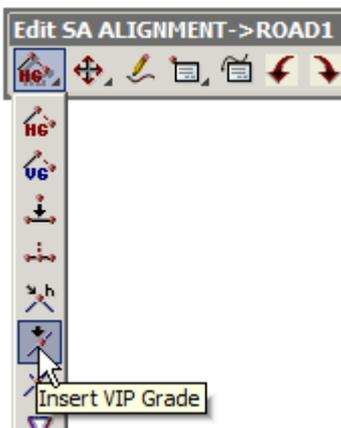
12d has many facilities to accurately place vertical geometry including typed input of grades and chainages. We are now going to insert a new IP point on the same grade as VIP 2 but 40 m from the intersection to allow us enough room to place a vertical curve. To do this we click on **Add/Remove IPs => Insert VIP Grade**.
