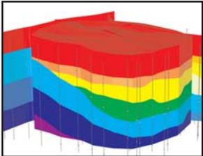
Define geologic model from boreholes and cross-sections
